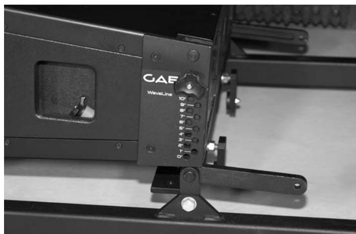
Now the front connection mechanism can be lowered without tilting. The mechanisms must be inserted precisely into each other. Make sure that the pins and forks are free of dirt.
