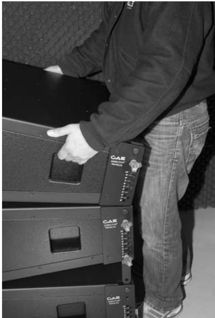
Load the first element to be mounted flush with the rear edge to the lower element.
