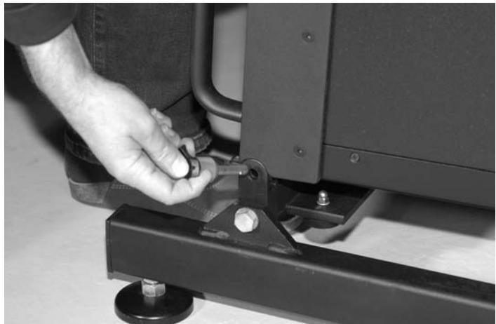
The ball lock pins must be fully inserted and flush against the mechanics surface, the release button must be completely jumped back. The disengaging of the locking balls can be checked visually.
