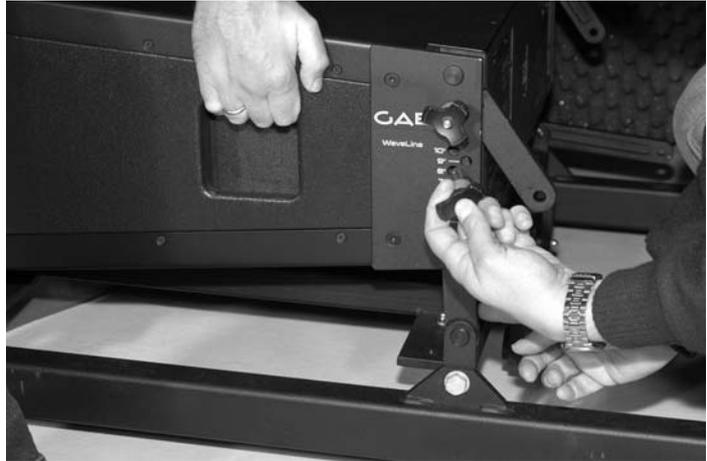
Lock the rear flight mechanics on both sides with the corresponding ball lock pins. By pressing the centric button the securing of balls is released and the pin fits into the bore.
