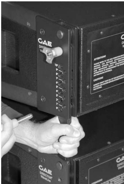
If the upper linking sword is not swung out, only the 0° position can be chosen. This can simplify and accelerate the dismantling within the flight case.
