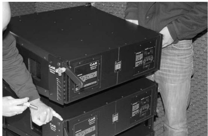
**⚠** At this situation coordinate yourself with the helping person unmistakably. Accidental or premature lowering of the element can cause serious injury to hands and fingers of the adjusting person! Only when the ball lock pin is securely
