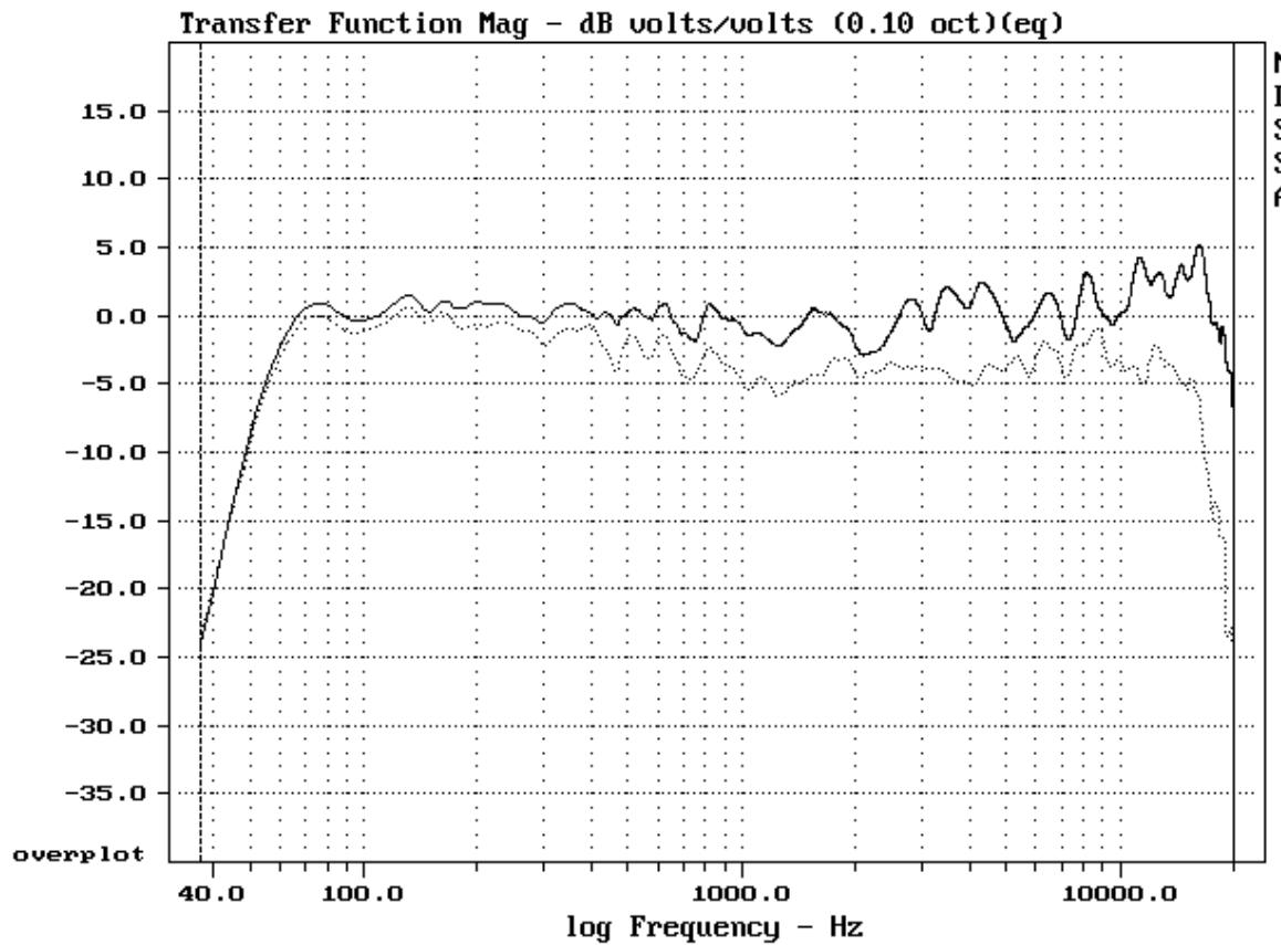
GAE System 10CX Frequency Response with Setup <System 10CX FR>
