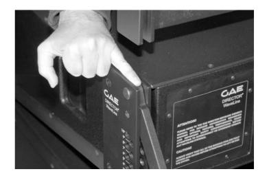
Make sure that the linking swords and mechanisms are free of dirt.
