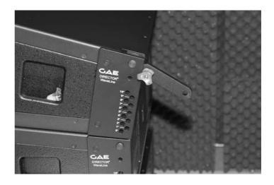
While the second person holds the element in the raised position, the first person can swing out the lower linking sword.
