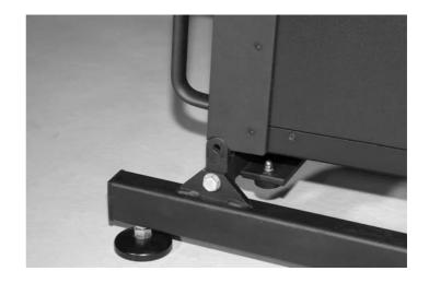
Lock the front flight mechanics on both sides with the corresponding ball lock pins. By pressing the centric button the securing of balls is released and the pin fits into the bore.
