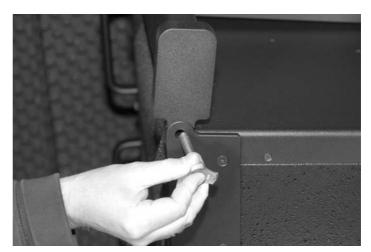
While the first person holds the flying cradle's rear end (outrigger) lifted, the second person now removes the upper in the park position located ball lock pin of the upper element and swings out the linking sword.
