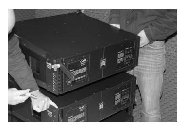
At this situation coordinate yourself with the helping person unmistakably. Accidental or premature lowering of the element can cause serious injury to hands and fingers of the adjusting person! Only when the ball lock pin is securely
