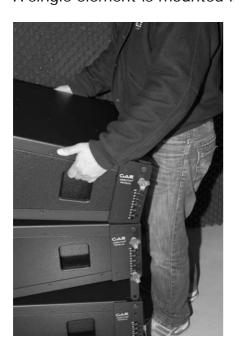
Load the first element to be mounted flush with the <u>rear</u> edge to the lower element.
