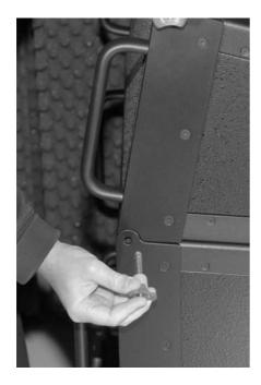
Lock the front flight mechanics on both sides with the corresponding ball lock pins. By pressing the centric button the securing of balls is released and the pin fits into the bore.
