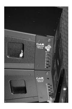
The elements are now at flush. Now remove the upper in the park position located ball lock pin of the lower element. You can store them in the handle of the upper element.
