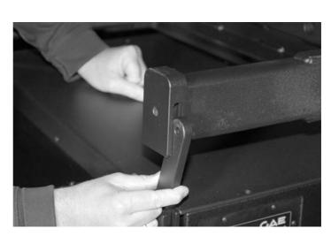
The ball lock pin must be fully inserted and flush against the mechanics surface, the release button must be completely jumped back. The disengaging of the locking ball can not be checked visually at this point, since the pin disappears in the flight mechanics. Procedure on the opposite side in the same way.
